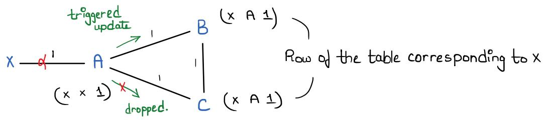
The X-A Link failure triggers an update from A to B and C. Now, assume that the update never reaches C as the signal is lost. The respective rows would be
