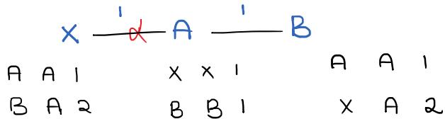
In the above example, the failure of X-A link triggers an update  $(X, \infty)$  from A to B. Suppose that B sends a periodic update  $(X, 2)$  to A before the triggered update is received. This would cause A to wrongly think a path B-X of Length 2 exists, which it updates in its table. B receives the triggered update and puts  $(X, \infty)$ .
