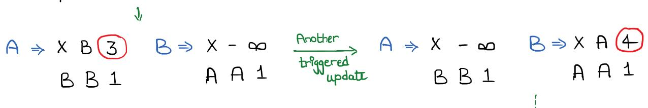
As the rows of A, B have changed; another update pair similar to above is triggered. This would inturn cause the cost (highlighted in red) to count upto  $\infty$ . (Hence the name)
